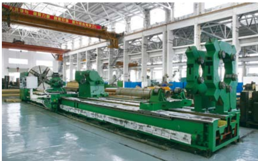
12m 40 t Ø2.5 m CG61200重型车床
